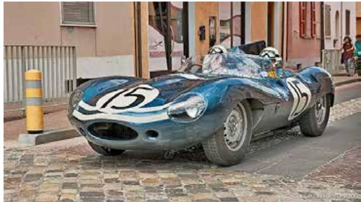
The Jaguar D-Type, produced from 1954 to 1957, was a highly successful race car (winning Le Mans in 1955, 1956, and 1957) based on the roadgoing C-Type, but with significant structural and aerodynamic design differences. The D-Type used the 3.4-liter, twin-cam, inline-6 engine that powered both the XK120 and the C-Type. Although the mill that produced between 160 and 180 horsepower made the XK120 the fastest production car in the
