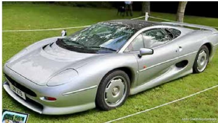
Jaguar's initial design for the XJ220, unveiled at the British International Motor Show in 1998, proposed a racing car with four-wheel-drive and V12 appropriate for FIA Group B racing. However, the sports car manufacturer's principal competitors, Porsche with its 959 and Ferrari with the F40, had already implemented compact, turbocharged engines that produced more power with less weight.
