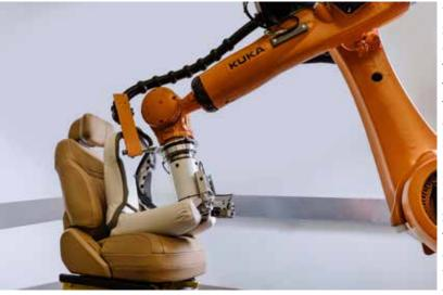
to ensure the heated seat is robust and will remain operational throughout a vehicle's lifespan. After all, you don't want to end up with a broken seat and a cold backside at that crucial moment in the winter!
