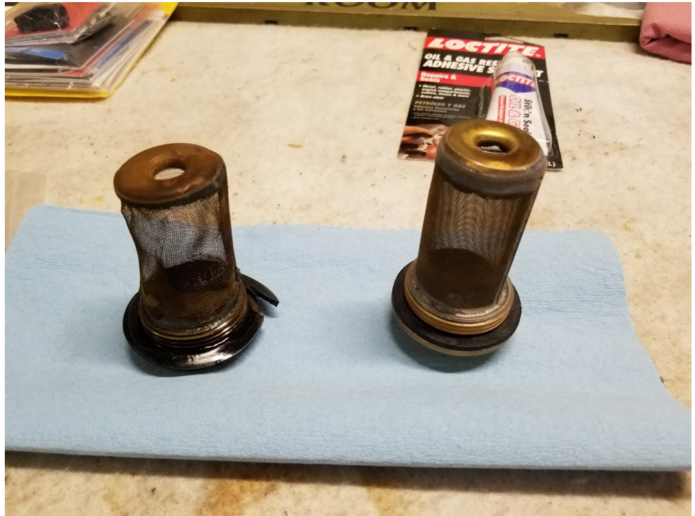
A side by side of the new and old drain plug and its integrated brass mesh filter.
